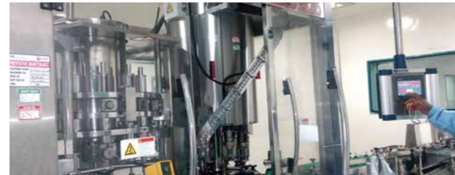
The high-speed Visco-bloc filling and capping machine at the Oral Liquids Section can fill up to 120 bottles per minute.
