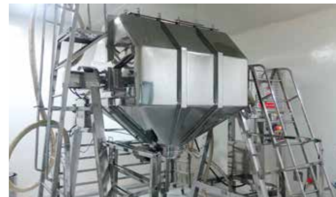
The 2500L Octagonal Blender at the Blending Section is fitted with an automated powder suction system that enables the operator to automatically load the powder.
