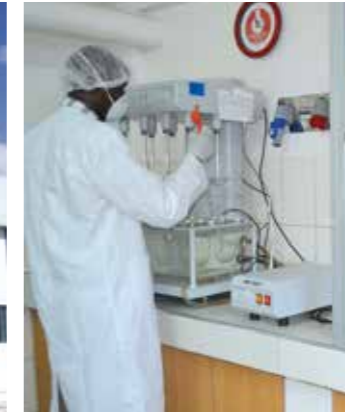
The wet chemistry laboratory where a QC Analyst collects samples from each jar of the dissolution test apparatus.
